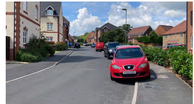
Figure 133. Waterers Way: Informal footway parking along the street reduces available effective width for pedestrians.
